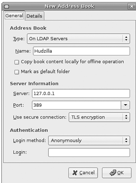
FIGURE 22.1 Configuring Evolution to use LDAP for addresses is easy for anonymous connections.
