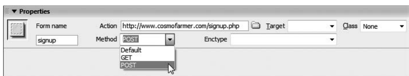
Figure 11-3: You'll generally want to use the POST method of sending data to the server. See step 7 for more details.
