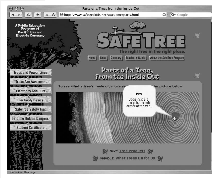
Figure 13-17: Using Dreamweaver's Show-Hide Elements behavior, you can make elements appear and disappear. In this example, several elements lay hidden on the page. When a visitor moves the mouse over different parts of the tree cross-section, informative graphics (each placed in a hidden element) suddenly appear. Moving the mouse away returns the element to its hidden state. Notice how the information bubble overlaps the tree image and the text above it—a dead giveaway that this page uses absolutely positioned divs.
