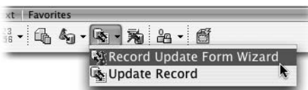
Figure 24-5: The Update Record menu's wizard can create a no-frills Update Record Form.
