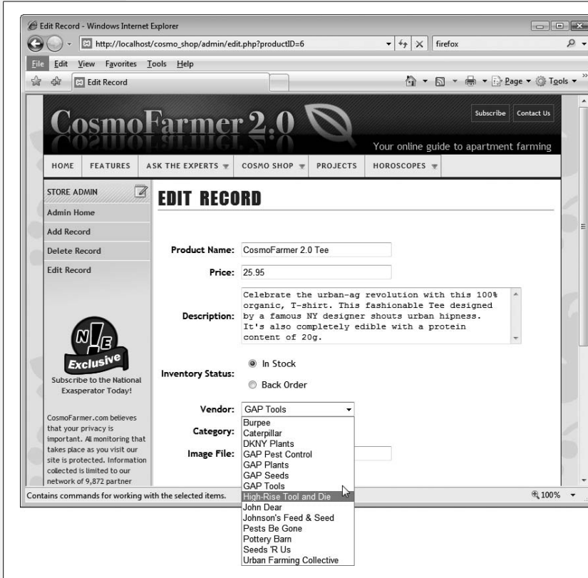
Figure 24-9: Dynamic form fields come in handy with update forms. Form fields are already filled out with database information that's ready to be edited. Menus can also be dynamically generated from records in a recordset. In this case, the menu (shown open) lists records retrieved directly from a database table containing the product categories for the CosmoFarmer online store.
