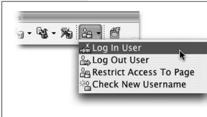
Figure 25-1: Dreamweaver provides access to all user-authentication server behaviors from the Application tab of the Insert bar.
