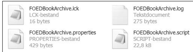
Figure 15-13. The HSQLDB is represented by simple TXT files
