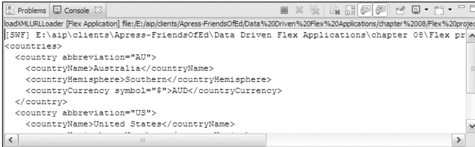
Figure 8-3. The toXMLString method provides a string representation of an XML object.
