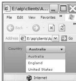
Figure 6-2. The ComboBox and Label controls populate from an external text file using variable pairs.
