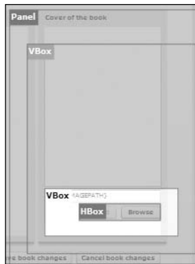
Figure 16-5. Container structure of the third panel
