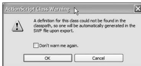
Figure 1-11. This warning lets you know that no class was found and so one will be created behind the scenes upon compiling.
