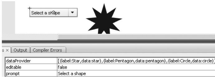
Figure 9-15. An array of objects defines the labels and data that populate a ComboBox.
