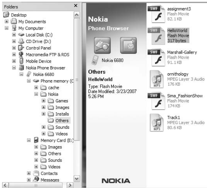
Figure 12-15. It is as simple as a drag-and-drop operation to get the SWF from the computer into the phone.
