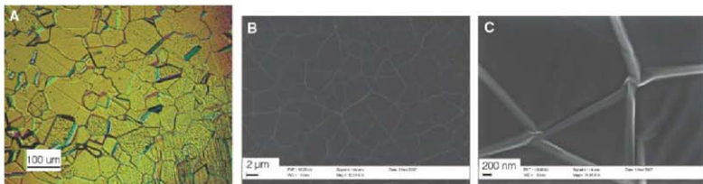
Fig. 1. (A) Optical images of Ni, and SEM images of (B) ^{13}\text{C} -labeled synthetic graphite and (C) the wrinkles.
