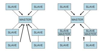
Fig. 5. Clock synchronization between nodes
