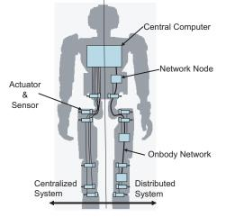
Fig. 1. Configurations of self-contained robots
