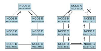
Fig. 4. Route reconfiguration(RM:Relay Mode, TM:Through Mode)
