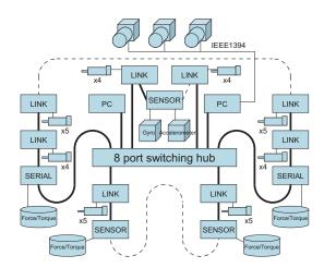
Fig. 12. Configuration of onbody network on HRP-3P
