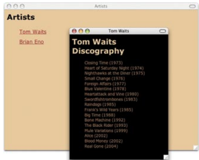
Figure 6-12. JavaScript allows you to open a window at a specific pixel size.
