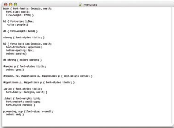
Figure 13-21. External style sheets contain only CSS rules and comments in a plain text document.
