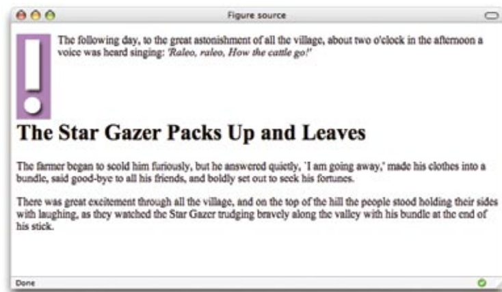
Figure 15-7. Clearing a left-floated element
