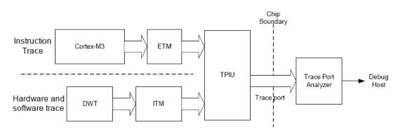
Figure 8. The Cortex-M3 Trace System
