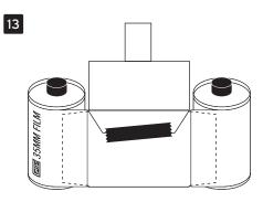
After sliding the cardboard tabs into the film canisters, wrap the top of the box over the back and tape it down. This should secure the entire box.
