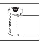
Light-safety is created by sandwiching the film between two layers of cardboard, and inserting those layers into the already light-safe film canister. Carefully slide both tabs into the film canister, taking care to push the canister snugly against the frame.
