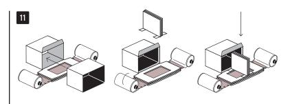
Insert the light tub it into the box, and add the light-splitter.
