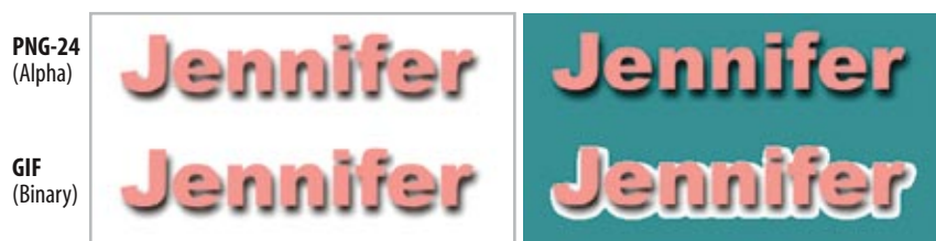
Figure 18-25. The difference between binary and alpha transparency becomes very clear when the background color of the page changes.
